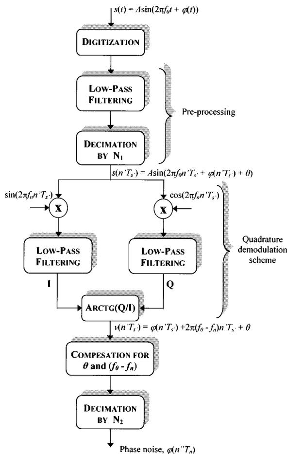
Fig. 1. Block diagram of the proposed method.
