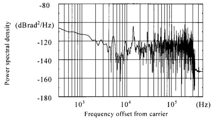
Fig. 6. Power spectral density of the phase noise affecting a 1 MHz sinusoidal carrier provided by a Philips model PM 5193<sup>TM</sup> function generator.
