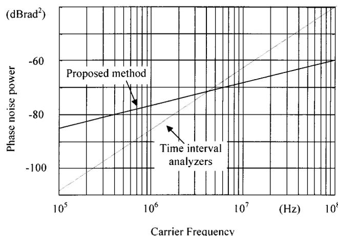
Fig. 4. Performance of the proposed method is compared to the typical one offered by time interval analyzers.
