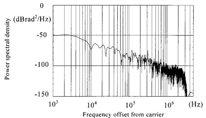
Fig. 7. Power spectral density of the phase noise affecting a 10 MHz sinusoidal carrier provided by a Philips model PM 5193<sup>TM</sup> function generator.
