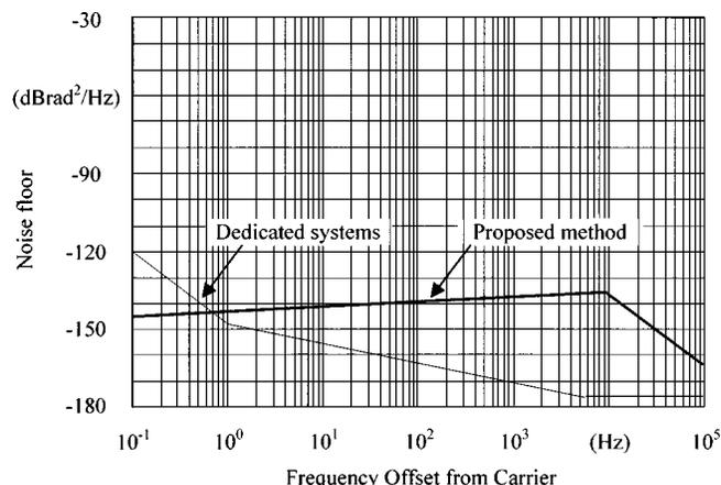
Fig. 3. Noise floor of the proposed method is compared to the typical one offered by dedicated systems.
