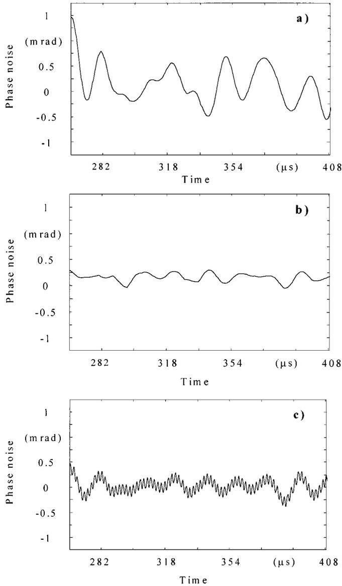
Fig. 2. Portion of the difference between measured phase noise and nominal one in the presence of a vertical resolution of the data acquisition system and a transition band of the low-pass filters in the quadrature demodulation scheme characterized respectively by (a) 8 bits and  $f_n/6$  extent, (b) 11 bits and  $f_n/6$  extent, (c) 11 bits and zero extent.
