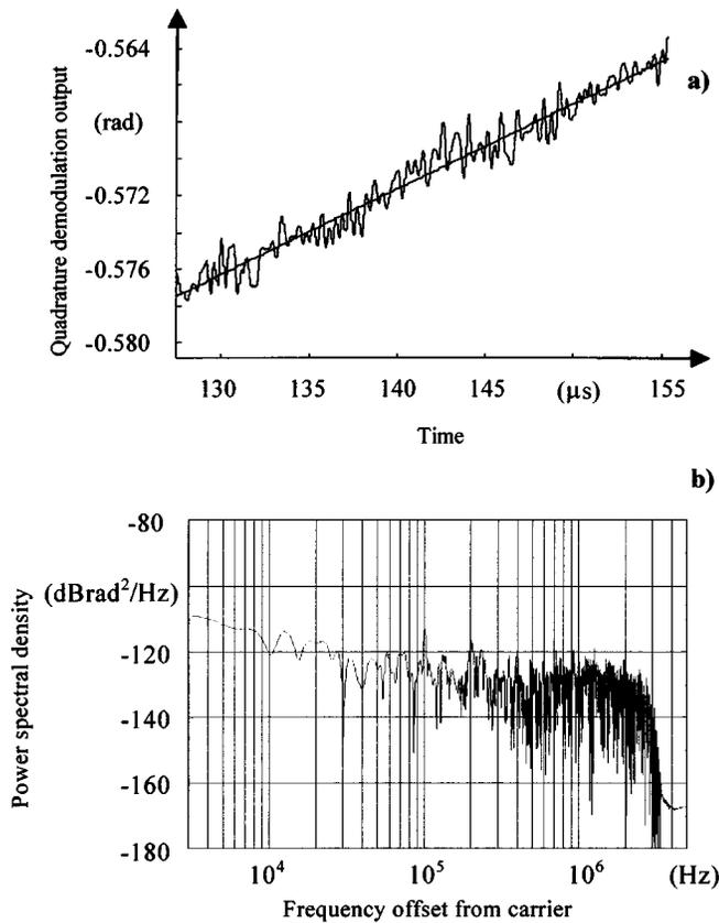
Fig. 5. (a) Measured phase noise affecting a 10 MHz sinusoidal carrier provided by a HP model 33 120A<sup>TM</sup> arbitrary waveform generator; (b) its power spectral density.
