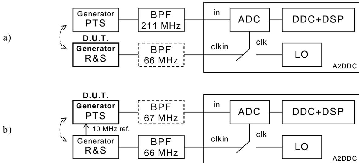
**Figure 1.** The high-frequency jitter measurement (a) and low-frequency phase noise measurement (b).
