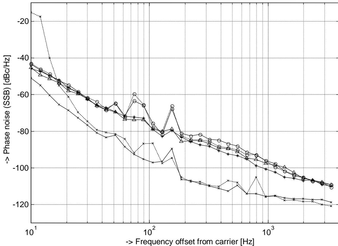
**Figure 2.** The low-frequency phase noise at various generator configurations. The analog input is 67 MHz and the clock is 66 MHz. The R&S and PTS (bundled) generator configuration represents ‘\*’ mark, the PTS (bundled) and R&S ‘Δ’, the PTS and LO ‘x’, the R&S and LO ‘o’. The filtered analog input is represented with a dashed line.
